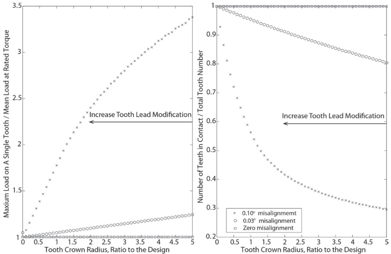
**Image 4:** Effect of crown radius on the spline tooth loads
