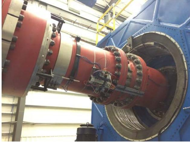
**Image 6:** Gear tooth coupling installed in NREL's 5-MW dynamometer facility.
