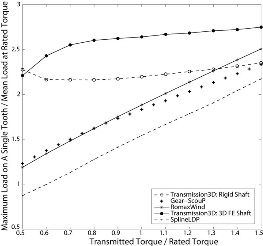
Image 3: Effect of torque on the maximum load of a single tooth
