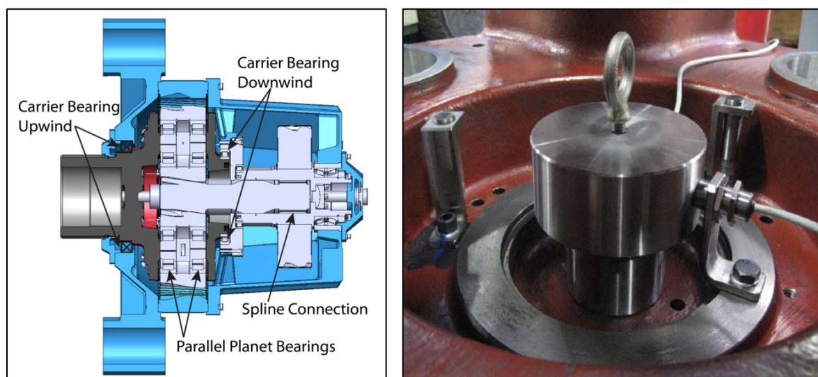
**Image 1:** A cutaway view of the GRC gearbox configuration (left) and one of two sun proximity sensors (right). *Photo by Edward Overly, NREL 26666.*
