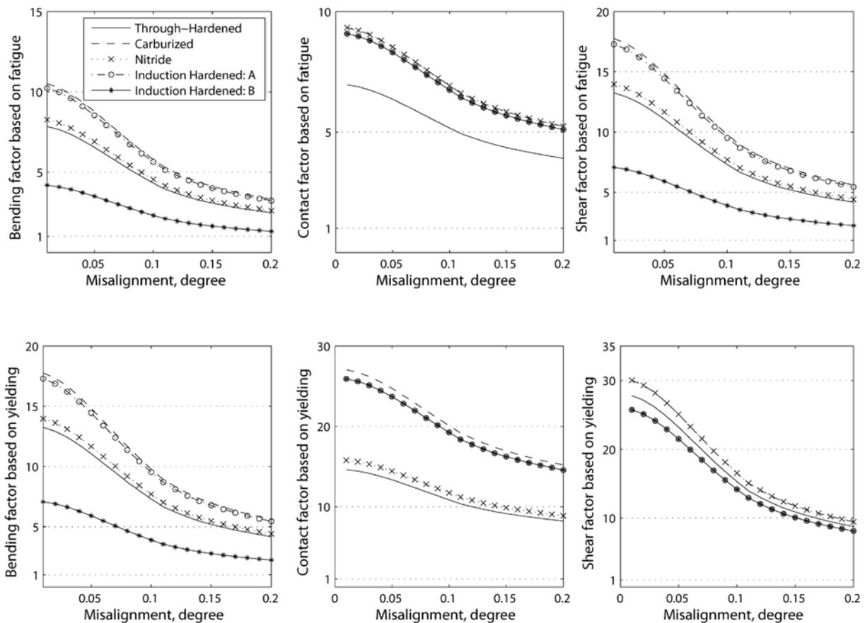
**Image 5:** Effect of heat treatment on fatigue safety factors
