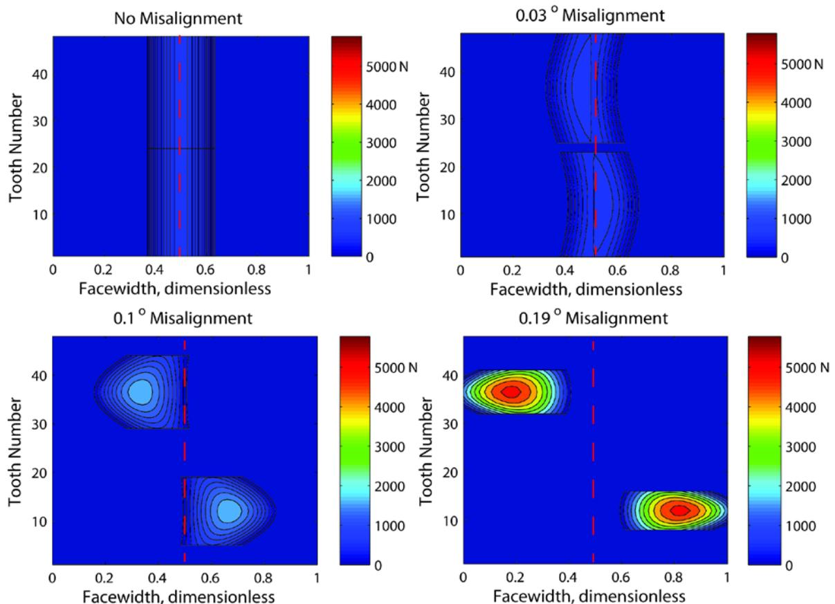
**Image 2:** Spline tooth load distributions calculated by the analytical model
