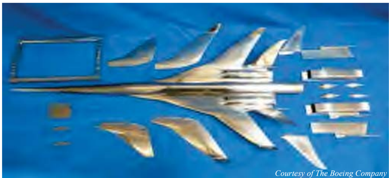
Figure 4-6. Photograph of Performance model and interchangeable parts
