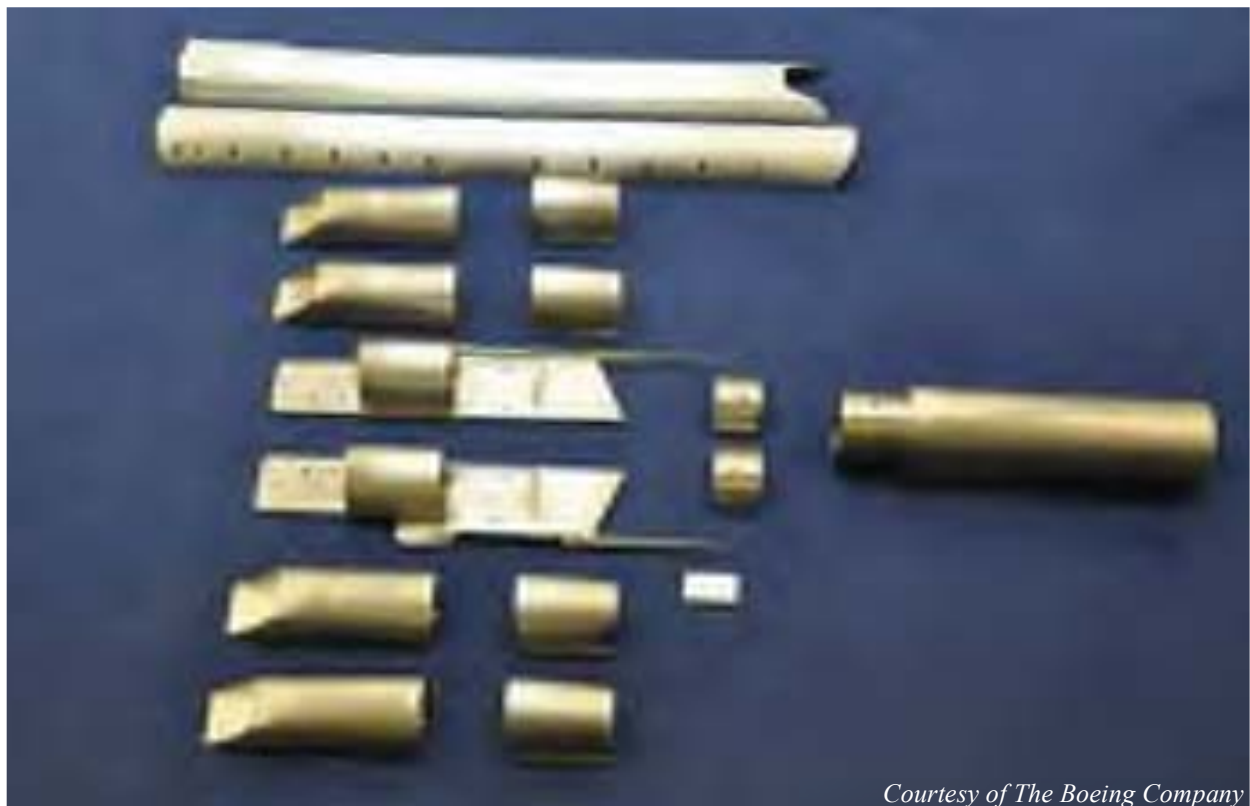
Figure 4-8. Photograph of Performance model new parts, and tailored sting covers
