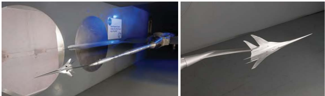
Figure 4–15. Photographs of Boom1 model with VS2 strut mounted in 9x7 wind tunnel
