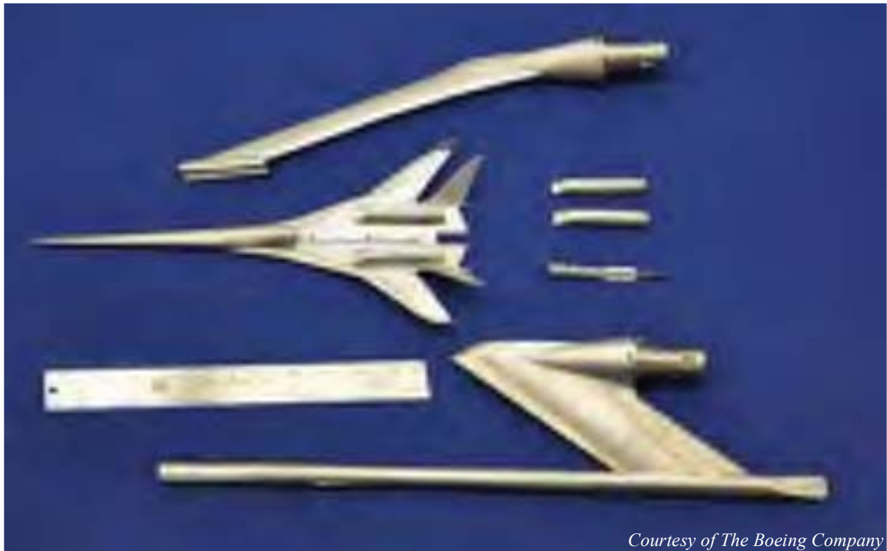
Figure 4–18. Photograph of Boom3 model, interchangeable parts, and VS3 and VS4 struts
