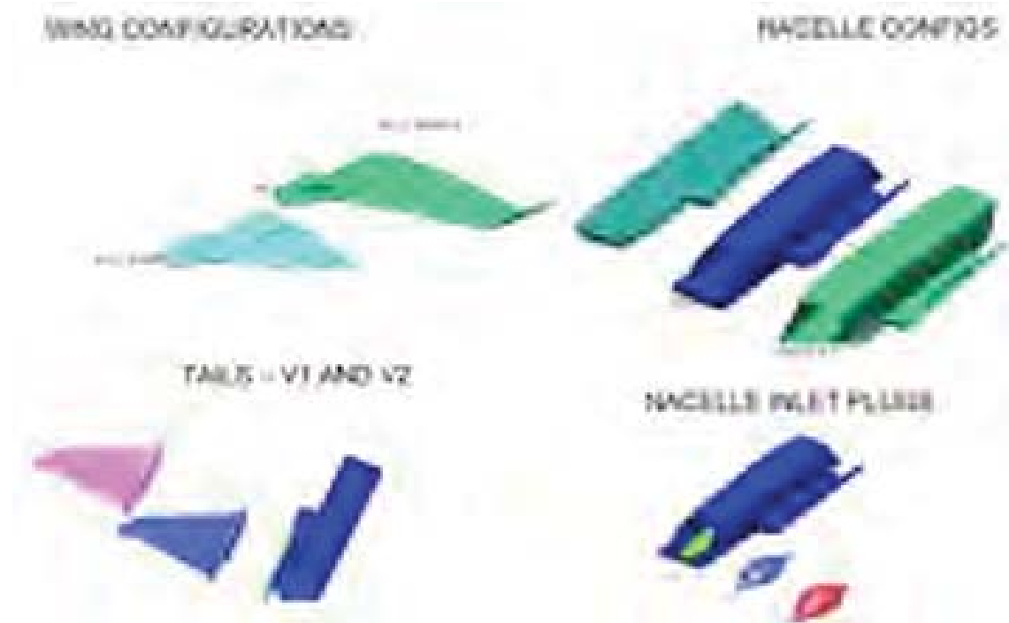
Figure 4-4. CAD views of Performance model modular parts
