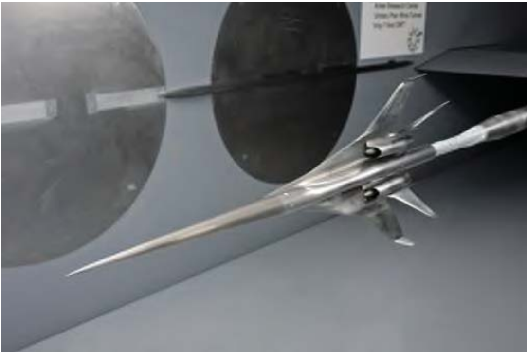
Figure 4–9. Boeing Performance model installed in Ames 9x7-ft wind tunnel
