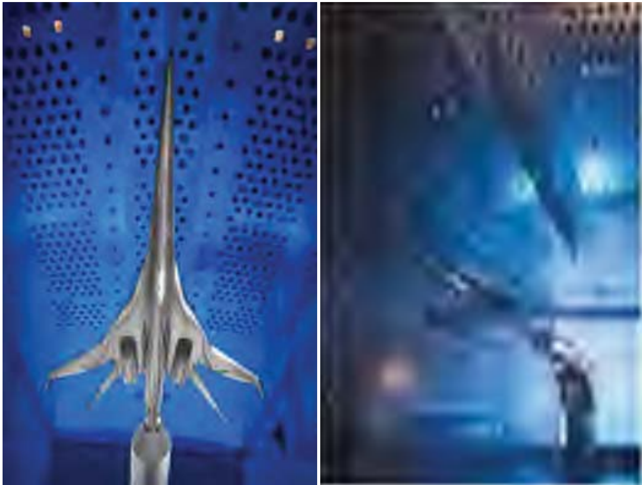
Figure 4-10. Boeing Performance model installed in Glenn 8x6-ft wind tunnel
