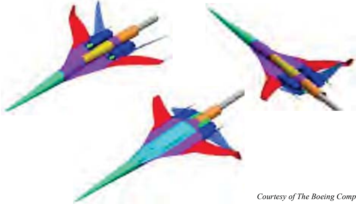
Figure 4-3. CAD views of Performance model components
