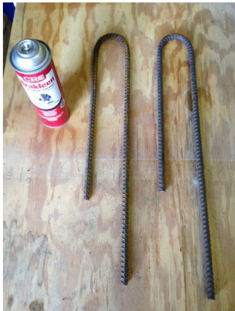
Figure 11. Using bent rebar for rebar installations has several advantages. It is more secure because the metal bar is anchored in two places. It also poses less safety risk for people who are wading through the stream because no sharp points protrude upward into the water column. This design was provided by Christopher M. Harbourt, Principal Engineer, Waterborne Environmental, Inc. Champaign, IL. www.waterborne-env.com . Installations are easier if one leg is a little longer than the other because you can start the longer leg first and then pound the rest into place.
