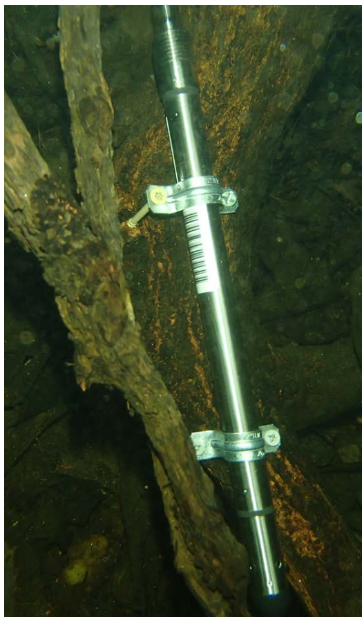
Figure 19. Some transducers come in a protective metal case and do not need to be encased in an additional housing.
