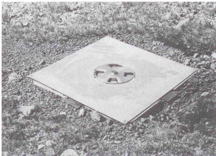
**Figure A1-4. A flush-mounted field mill for calibration**
