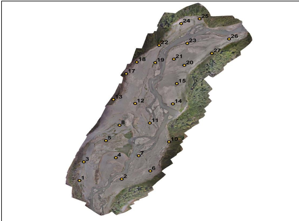
Figure 14. Photo identifiable points are selected from an existing orthomosaic image with elevation measurements from a LIDAR collection for input into the photogrammetric model.
