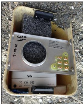
Figure 4. GoPro Hero2 integrated into the Raven nose cone.
