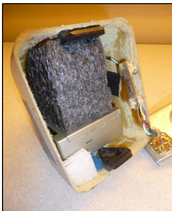
Figure 4. GoPro Hero2 integrated into the Raven nose cone.
