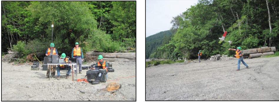
Figure 11. Field operations require minimal set up for ground station navigation (laptop and uplink/downlink antennas) with hand- launch and deep stall landing recovery of the small Raven UAS.
