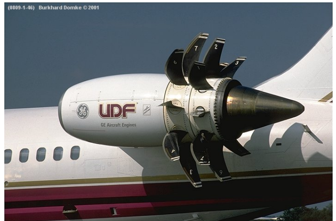
Figure 1.—Top: GE/NASA Unducted Fan (UDF) model installed in NASA wind tunnel (1985). Bottom: GE UDF engine demonstrator installed on the MD-80 testbed aircraft (1987). UDF had equal blade counts, eight each on the front and aft rotors.
