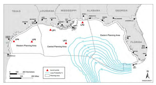
Figure A-1. Location of Five Hypothetical Oil-Spill Launch Points for OSRA within the Study Area. (Spatial variability of the Loop Current is from Vukovich [2007] and is shown as percent of time that the Loop Current watermass is associated with a particular location.)
