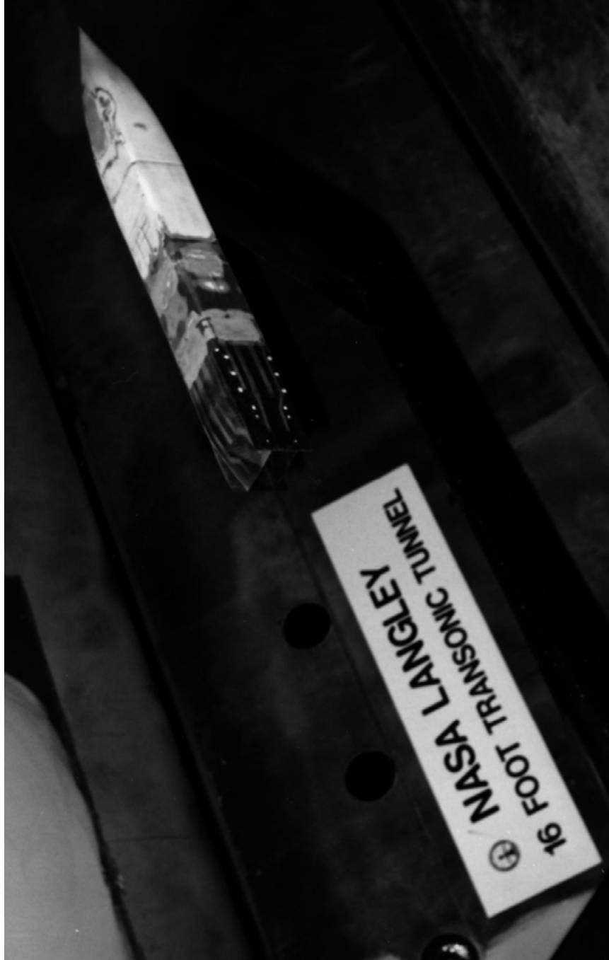
Figure 11. Model with nozzle N1 installed in the 16-Foot Transonic Tunnel.
