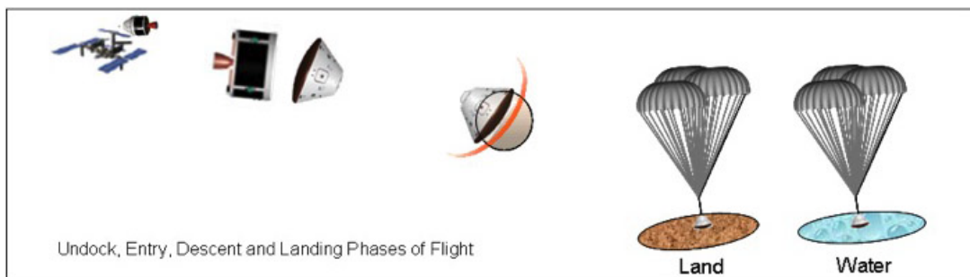
Figure 6.2-2. Phases of the Entry, Descent, and Landing Included in the Integrated Risk Assessment
