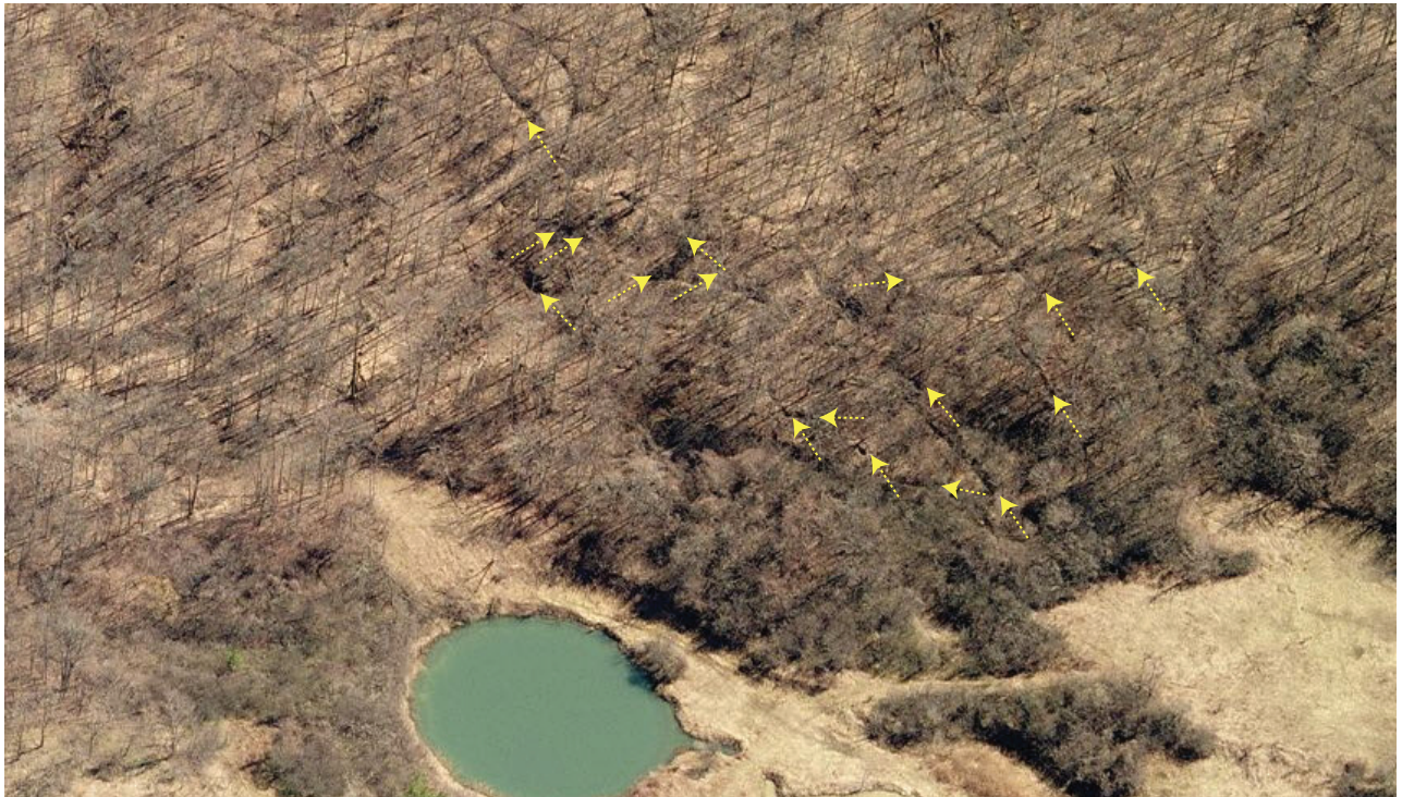
Figure 4. Major fractures above the Tully Valley brine fields: (A) near the north end of west brine field and (B) above the central sinkhole in the east brine field, Onondaga County, N.Y. (Arrows indicate location and orientation of large fractures on the lower hillside above each brine field.)
