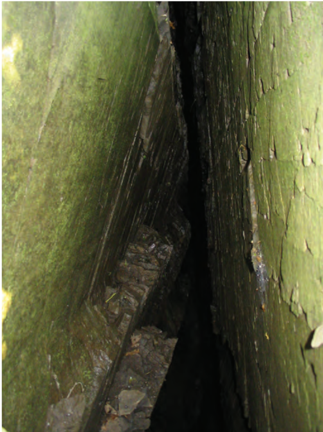
Looking downward into an open bedrock fracture which is about 30 feet deep. The left face has pulled away from the right face of the bedrock fracture in response to land-surface subsidence in the former brine field.
