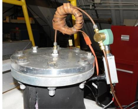
**Figure 6.** Air insertion line showing heating tape (to keep air from freezing upon injection) and solenoid for remote operation.
