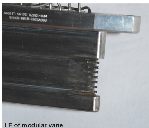
Figure 6.—Leading edge Kiel head instrumentation on main diffuser vane
