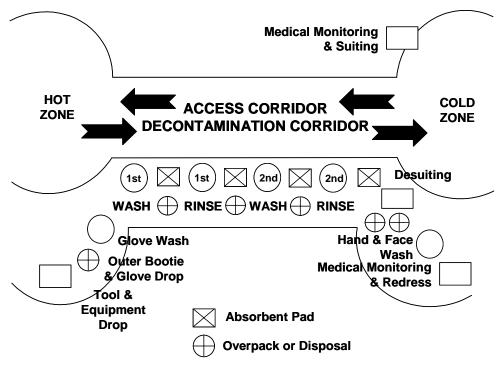
Figure 8-1 Access and Decontamination Setup
