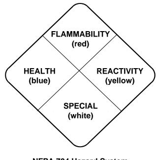
Within each diamond is a number from 0 to 4 indicating the hazard level in emergency situations. Zero indicates **no** hazard and 4 indicates a **major** hazard. For example, gasoline is listed as a 3 under flammability.
