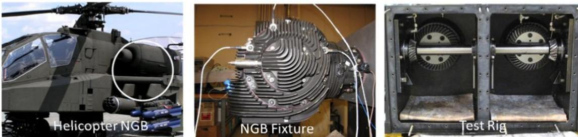
Figure 2.—Three spiral bevel geared systems.
