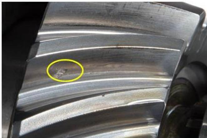
Figure 16.—Damage to one pinion tooth.
