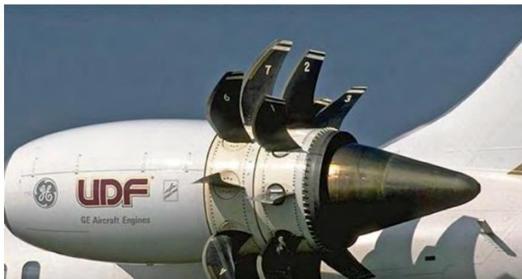
Figure 1.—General Electric (GE) unducted fan demonstrator.
