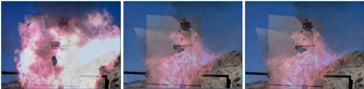
Figure 9.—Shape charge detonation, full-circumference configuration.
