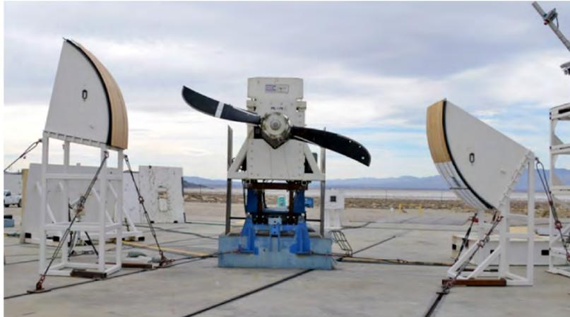
Figure 6.—Spin rig on T406 spin fixture.
