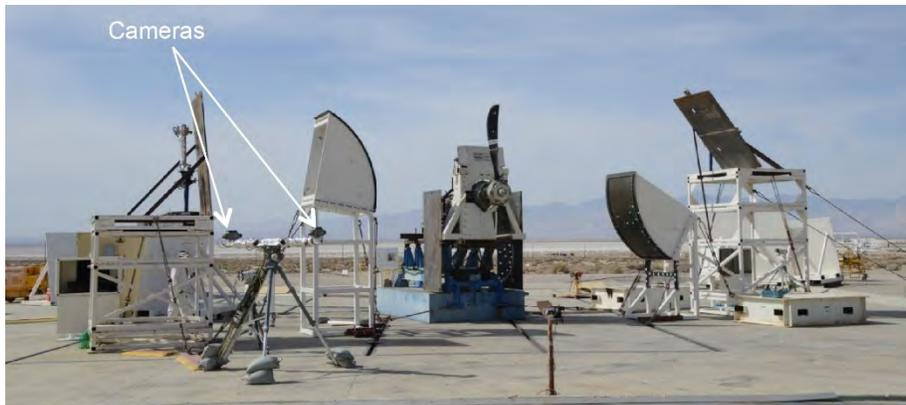
Figure 23.—Cameras used to measure blade kinematics.
