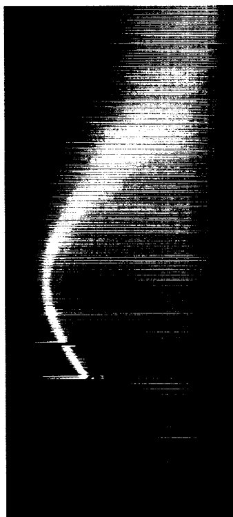
The spiral path of an electron beam around magnetic field lines can be seen clearly in this photograph taken in a plasma research chamber.
