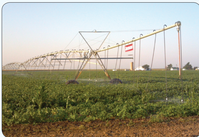
Center pivot irrigation system with drop nozzles in western Kansas, photograph taken by Lori Marintzer, U.S. Geological Survey.
