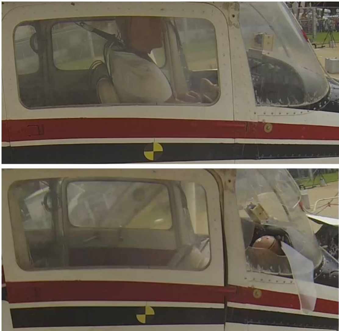
Figure 17 - Test 2 co-pilot head flail. Before impact (top) and max flail (bottom)
