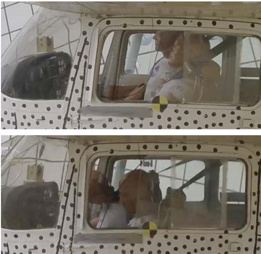
Figure 29 - Test 3 pilot head flail. Before impact (top) and max flail (bottom)
