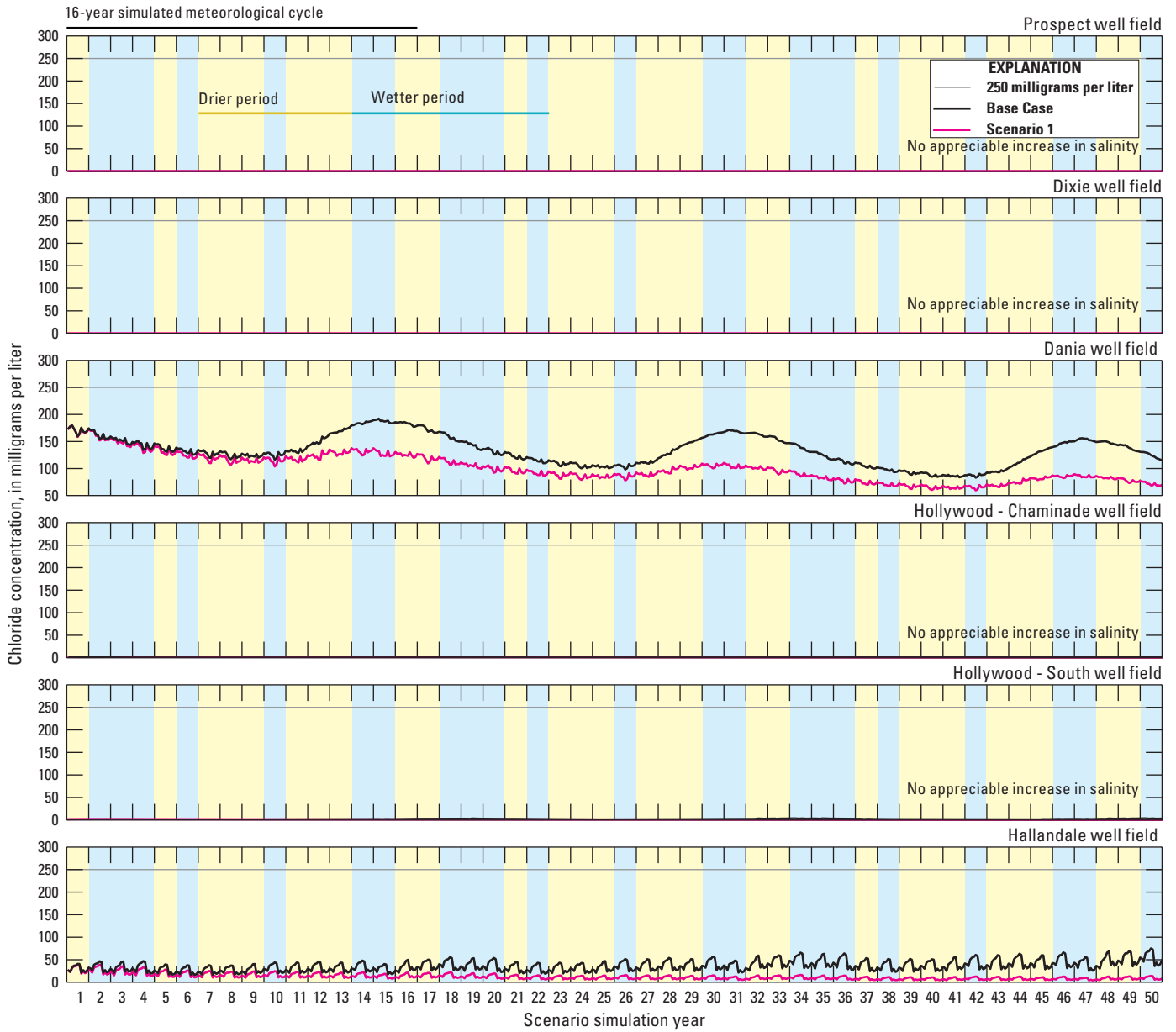
Figure 30. Simulated, flow-weighted, average chloride concentration at select well fields for the Base Case Scenario and Scenario 1. Yellow shading indicates drier than average climatic periods, and blue shading indicates wetter climatic periods, as shown by deviations from average rainfall in figure 27.
