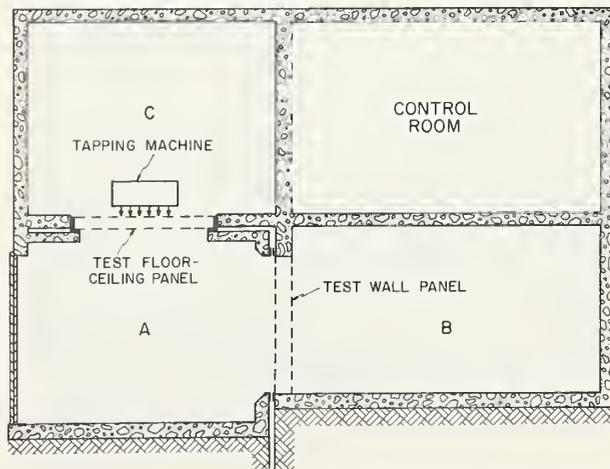
FIGURE 1. Vertical section of NBS sound transmission facilities.
