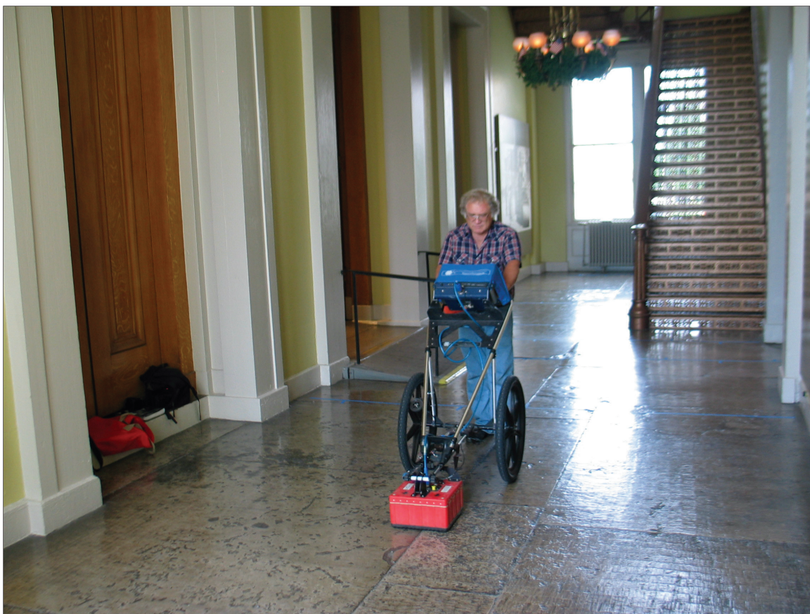
Figure 10. Conducting the ground-penetrating radar survey with the GPR cart and 400 MHz antenna in the North Transept geophysical project area (view to the west southwest).
