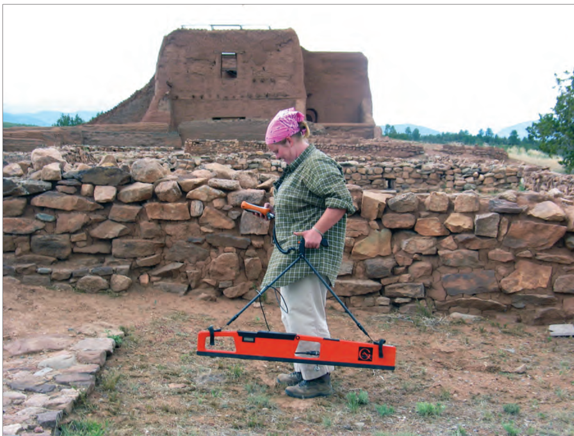
Figure 19. Demonstrating the use of the electromagnetic induction meter for conductivity surveying (view to the north).
