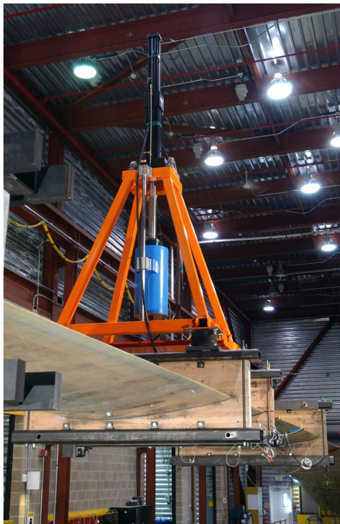
Figure 2. A prototype resonance fatigue shaker mounted on a 37-m blade at NREL. The blue mass is moved up and down relative to the blade using a hydraulic actuator mounted on top of the device.
