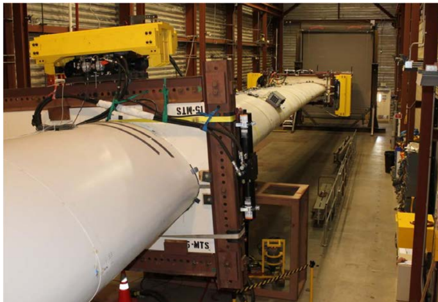
Figure 5. MTS IREXs installed on a turbine blade (viewed from root to tip) for conduction of a biaxial resonance fatigue test.
