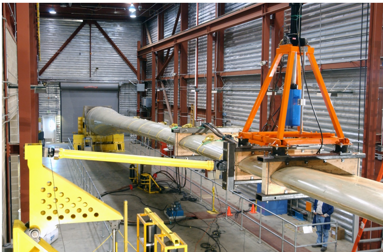
Figure 3. BREX fatigue test system combining a linear flap fatigue resonance shaker and a force-displacement lead-lag fatigue test.
