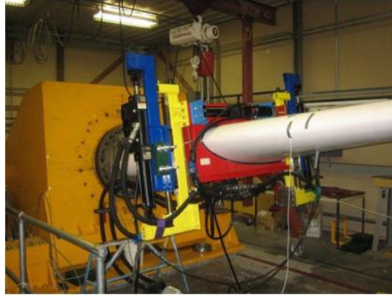
Figure 4. Prototype linear initial resonance excitation system in both the flap and lead-lag directions mounted on a 9-m blade.
