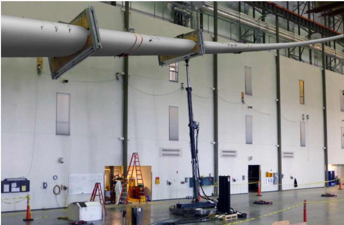
Figure 6. GREX 50 in operation on a flap fatigue test at the Wind Technology Testing Center.
