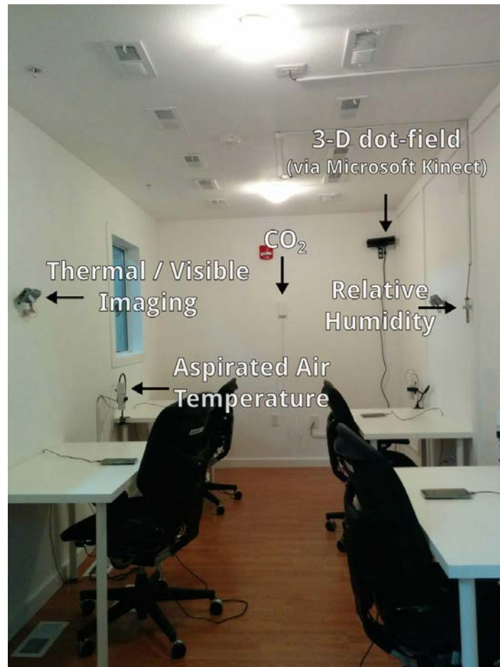
Figure 3. An image of the Comfort-Suite climate-controlled chamber configured as a simulated office environment; the positions of various sensors are annotated
