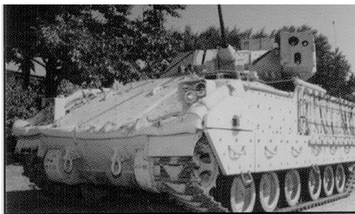
Bradley Fire Support Team Vehicle (BFIST) Provides artillery support and target acquisition by day or night.
