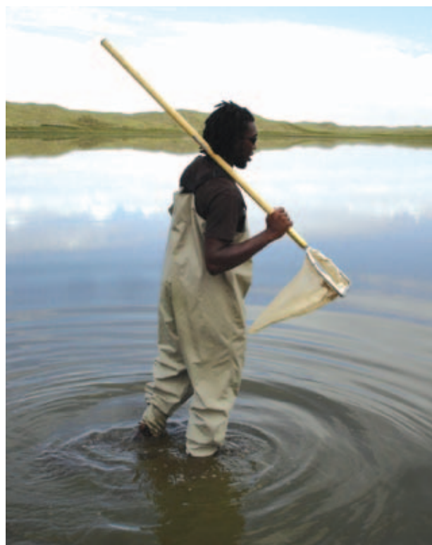
Sampling with a D-net for benthic macroinvertebrates. Photo courtesy of Great Lakes Environmental Center.
