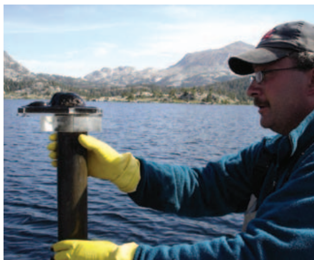
Retrieving a sediment core.
