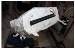
Figure 5. Urine Containment Bag, used for holding discarded UCDs until they can be disposed of along with other trash from ISS.
