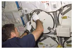
Figure 6. External view of a MELFI, showing the covers for the 4 dewars.
