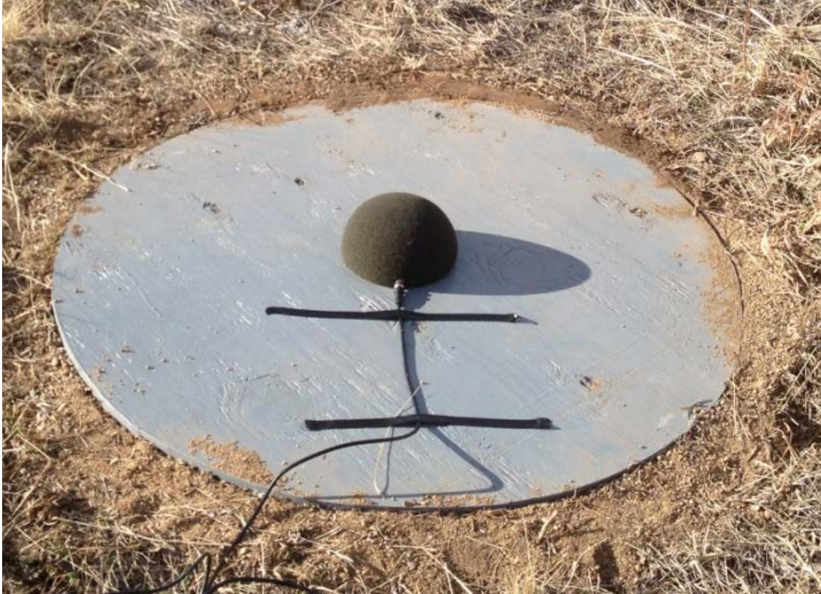
Figure A1. The sound board during the test (Photo by Jason Roadman, NREL)
