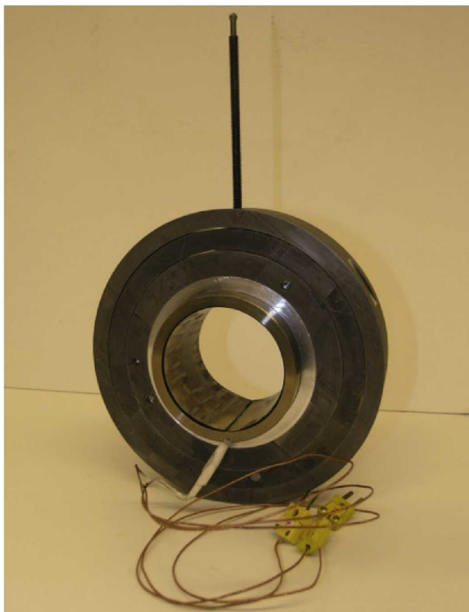
Figure 5.—Photograph of the test bearing with concentric dead weight loading rings and torque arm.
