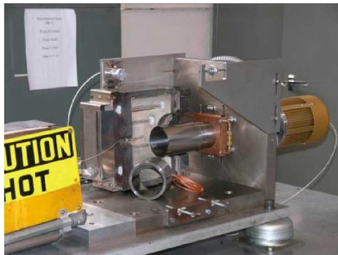
Figure 4.—Photograph of the test rig used for GE T700 bearing tests.
