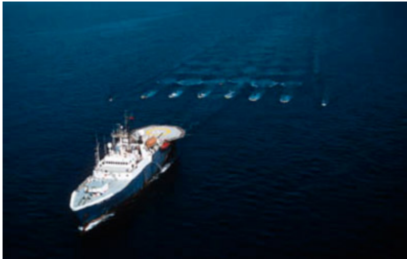
Figure 3. Marine seismic vessel towing multiple hydrophone streamers
