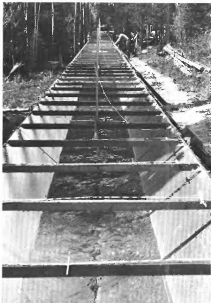
FIGURE 8.—View of Allenspark flume showing the triangular section. Point gages for measuring water-surface elevations were mounted on spacers crossing the flume. Readings were made with a level.
