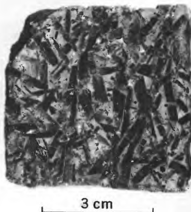
FIGURE 19.—Photograph of polished section from the drill core of the John Hay, Jr., well 1, depth 1,710 ft 4 in to 1,710 ft 6 in, showing large crystals of shortite.
