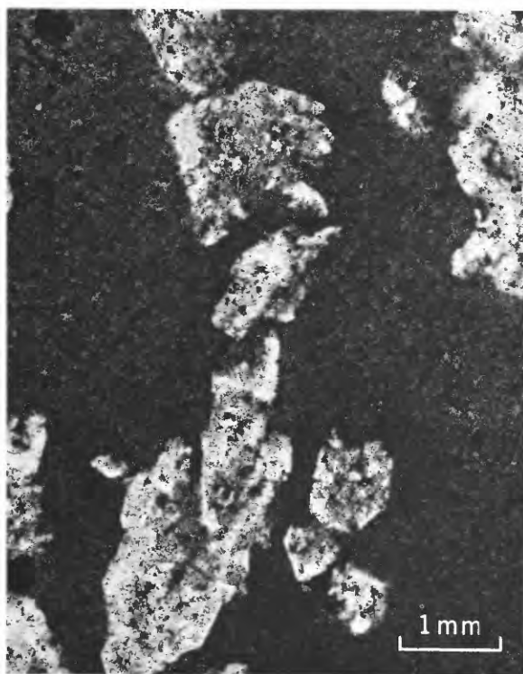
FIGURE 9.—Photomicrograph of thin section from drill core of the John Hay, Jr., well 1, depth 1,342 ft. 10 in., showing the sequence shortite to bradleyite. Plane-polarized light. \times 15 .
