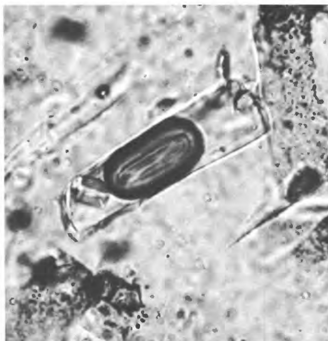
FIGURE 28.—Photomicrograph of the thin section of figure 26 showing liquid inclusion containing a gas and solid phase. Plane-polarized light. \times 800 .
