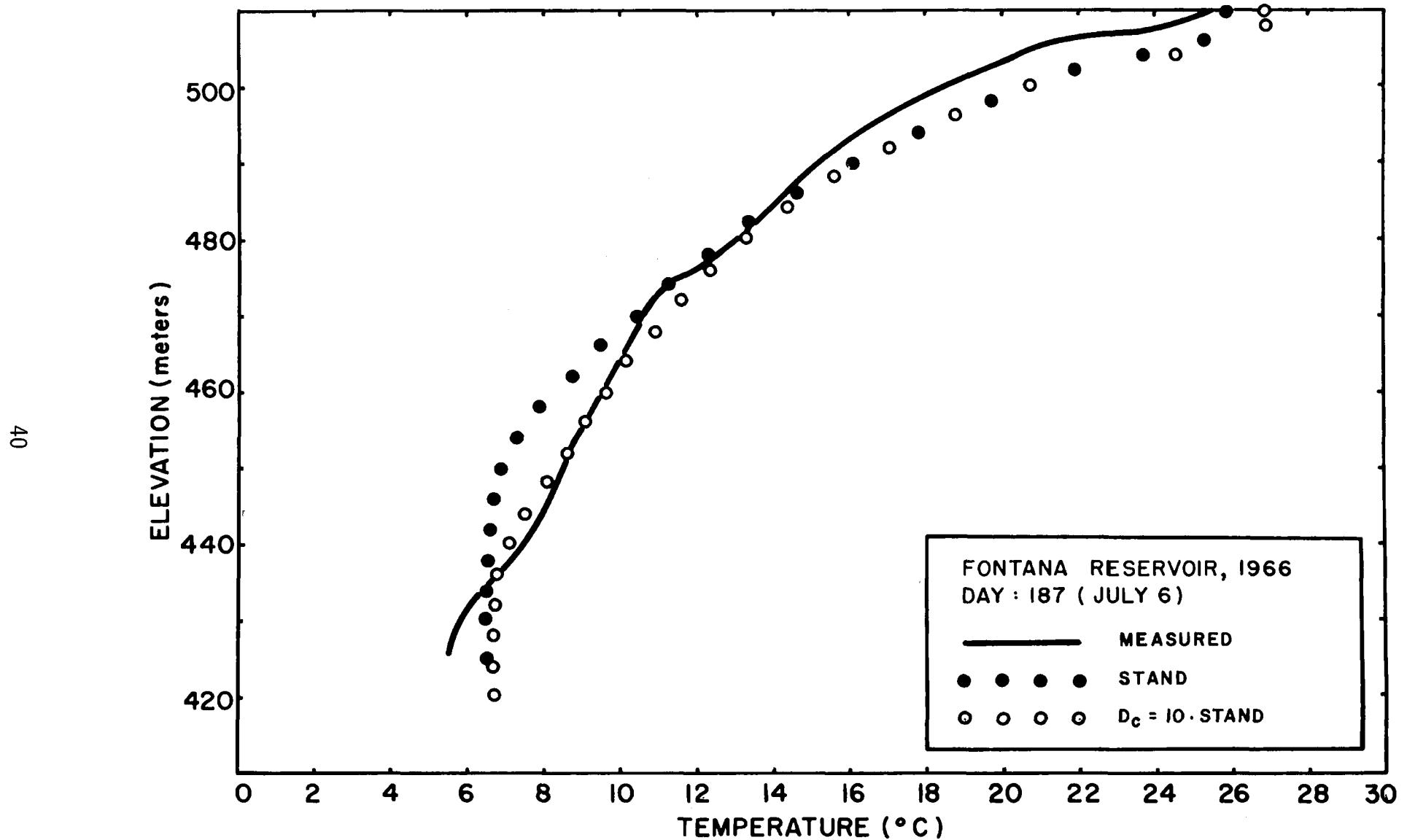
Figure 5. WRE model -- Effects of Diffusion Coefficient (July 6)
