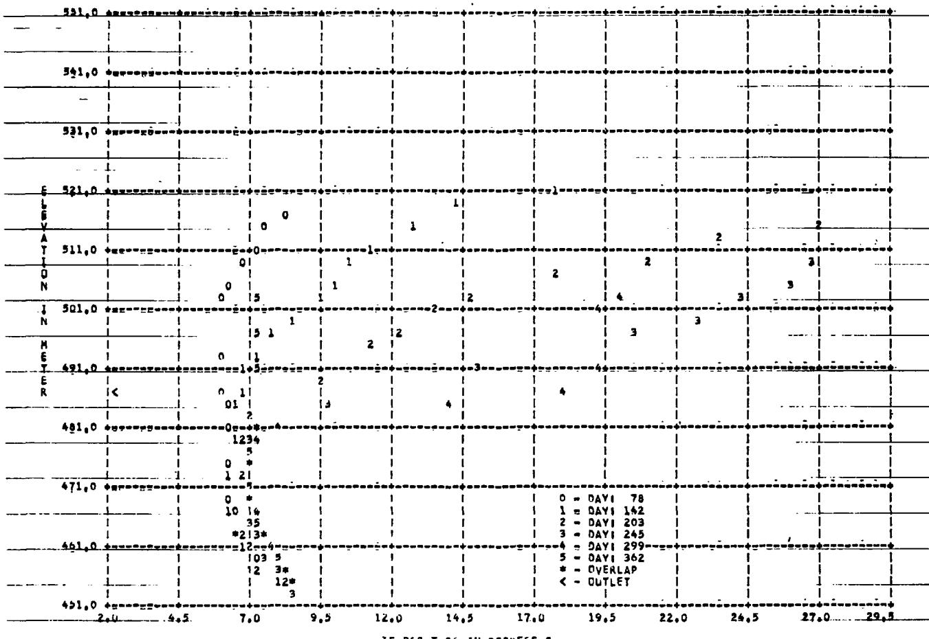
Figure 117 MIT MODEL \* SOUTHERN HOLSTON 1953--MEASURED TEMPERATURE PROFILE--
