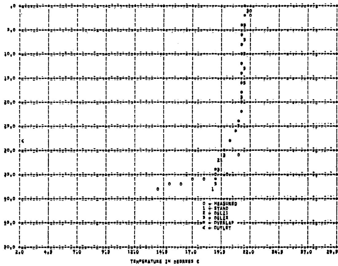
Figure 76 MJT MODEC - CHEROKEE RESERVOIR 1967- DAY 1277 SURFACE ELEV 319.1 M
