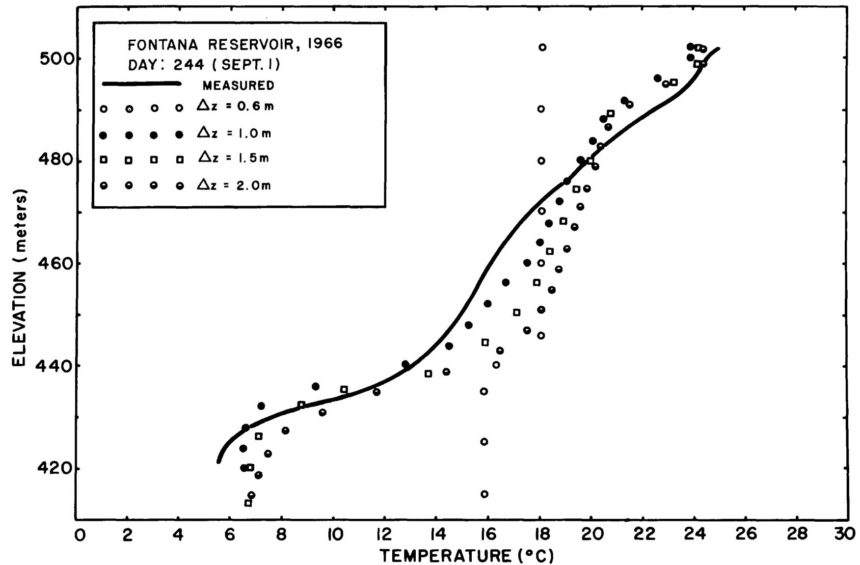
Figure 3. WRE model -- Effect of Thickness of Horizontal Layer (Sept. 1)
