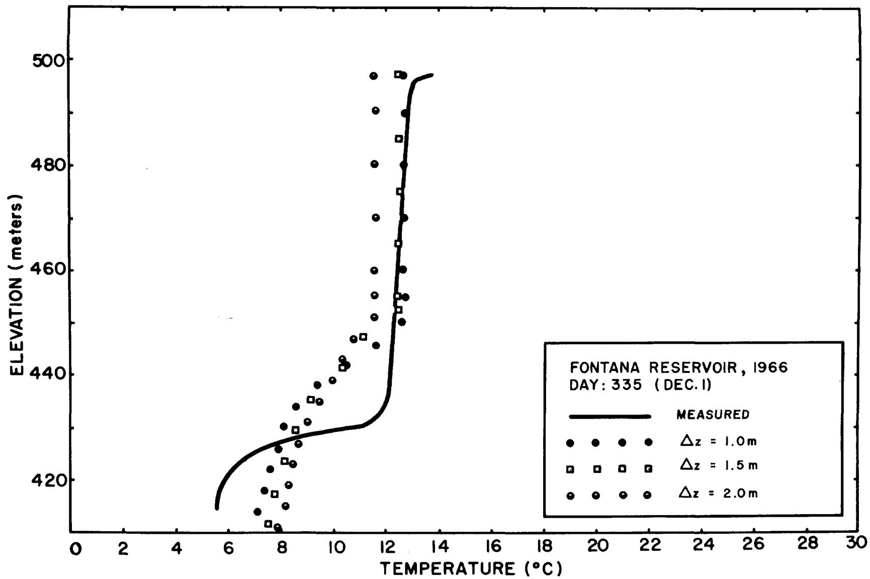
Figure 4. WRE model -- Effect of Thickness of Horizontal Layer (Dec. 1)
