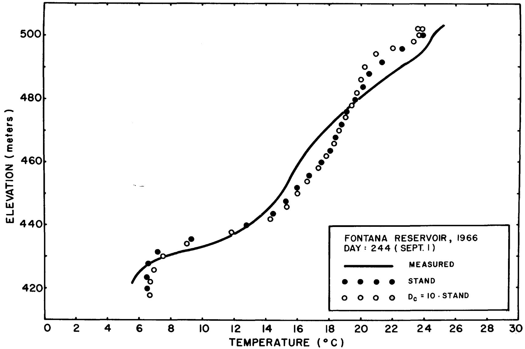
Figure 6. WRE model -- Effects of Diffusion Coefficient (Sept. 1)
