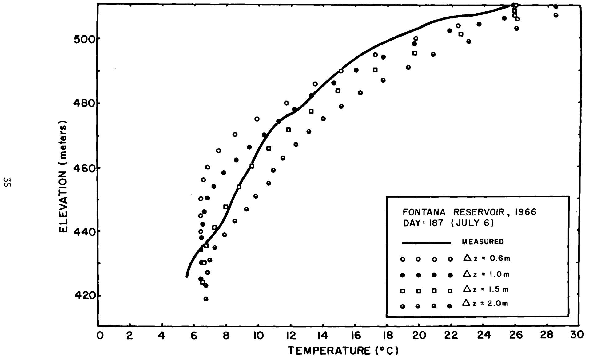
Figure 2. WRE model -- Effect of Thickness of Horizontal Layer (July 6)
