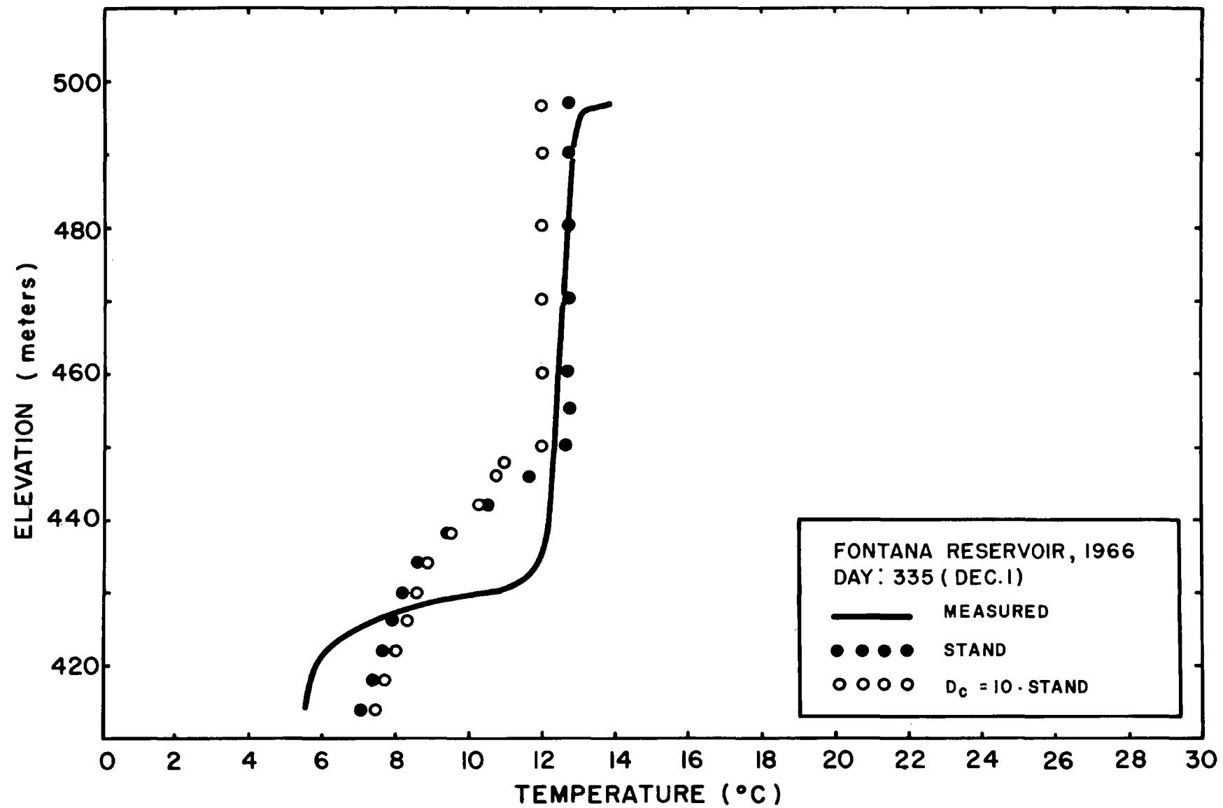
Figure 7. WRE model -- Effects of Diffusion Coefficient (Dec. 1)
