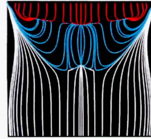
Fig. 14. Computed surface flow pattern for the inlet flow Mach number of 1.1 and incidence of 10.0 dg
