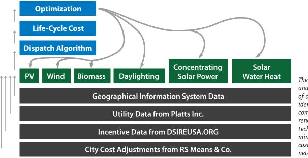
The REO tool analyzes a variety of data used to identify the optimal combination of renewable energy technologies needed to minimize the life-cycle cost of achieving the net-zero goal.
