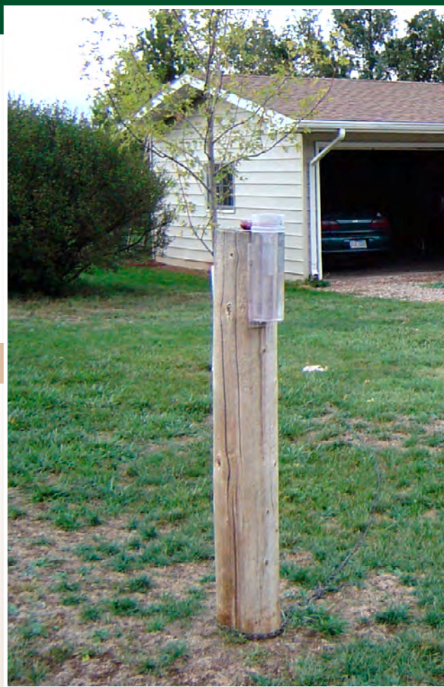
Photograph of 11-inch rain gage at a location west of Hermosa where 10.50 inches of precipitation was measured on August 17, 2007 (photograph by Robert D. Jarrett).
