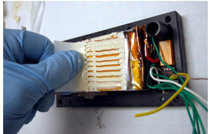
Figure 8.—Heat transfer/gap filler applied to exposed face of cell-pack.
