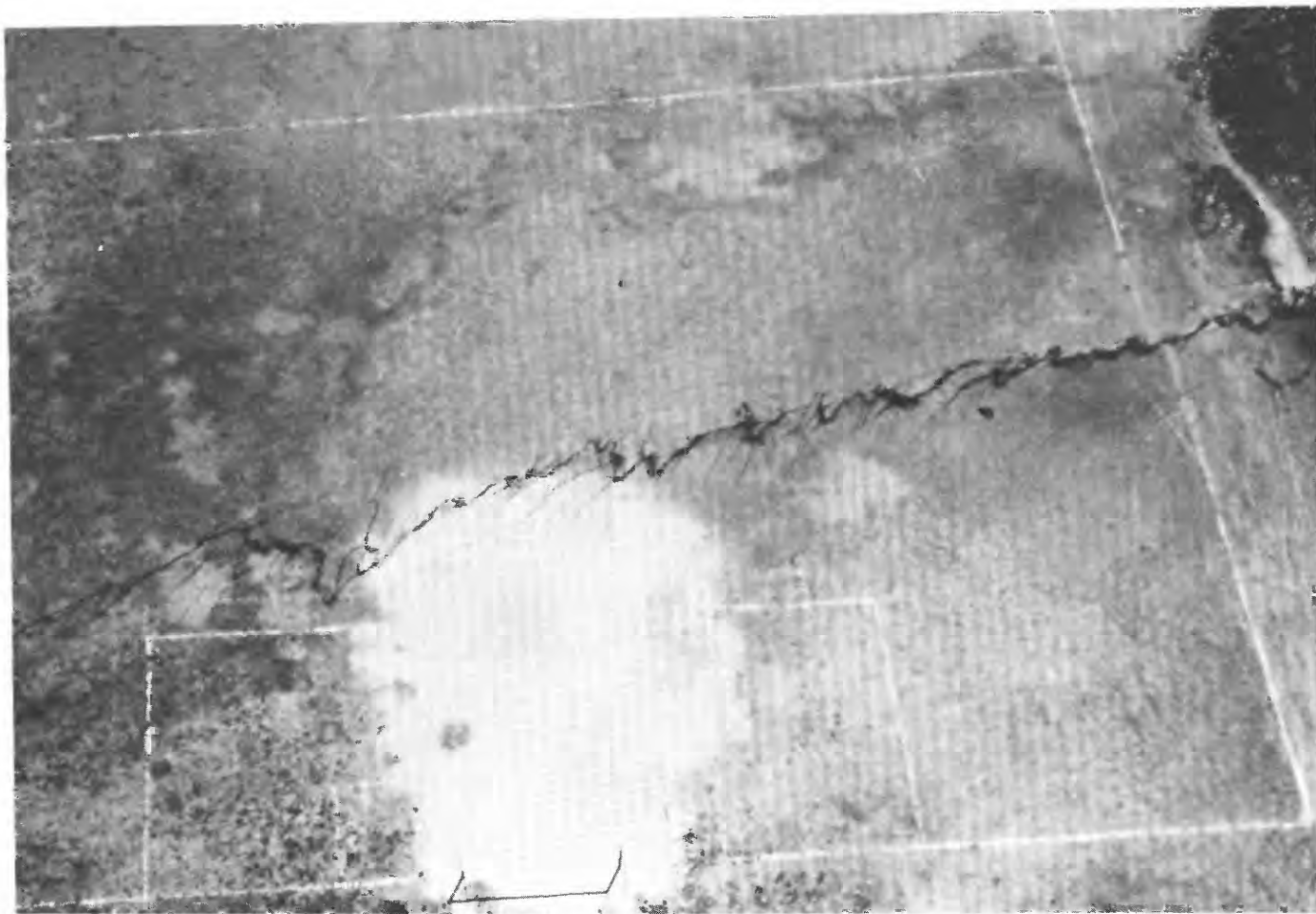
FIGURE 26.—Oblique aerial view of Motagua fault trace crossing a soccer field at Gualán (station 5, table 7). Note characteristic right-stepping en echelon fractures and sinistral offset (89 cm) of white sideline stripe at right. See figure 23 for location of Gualán.
