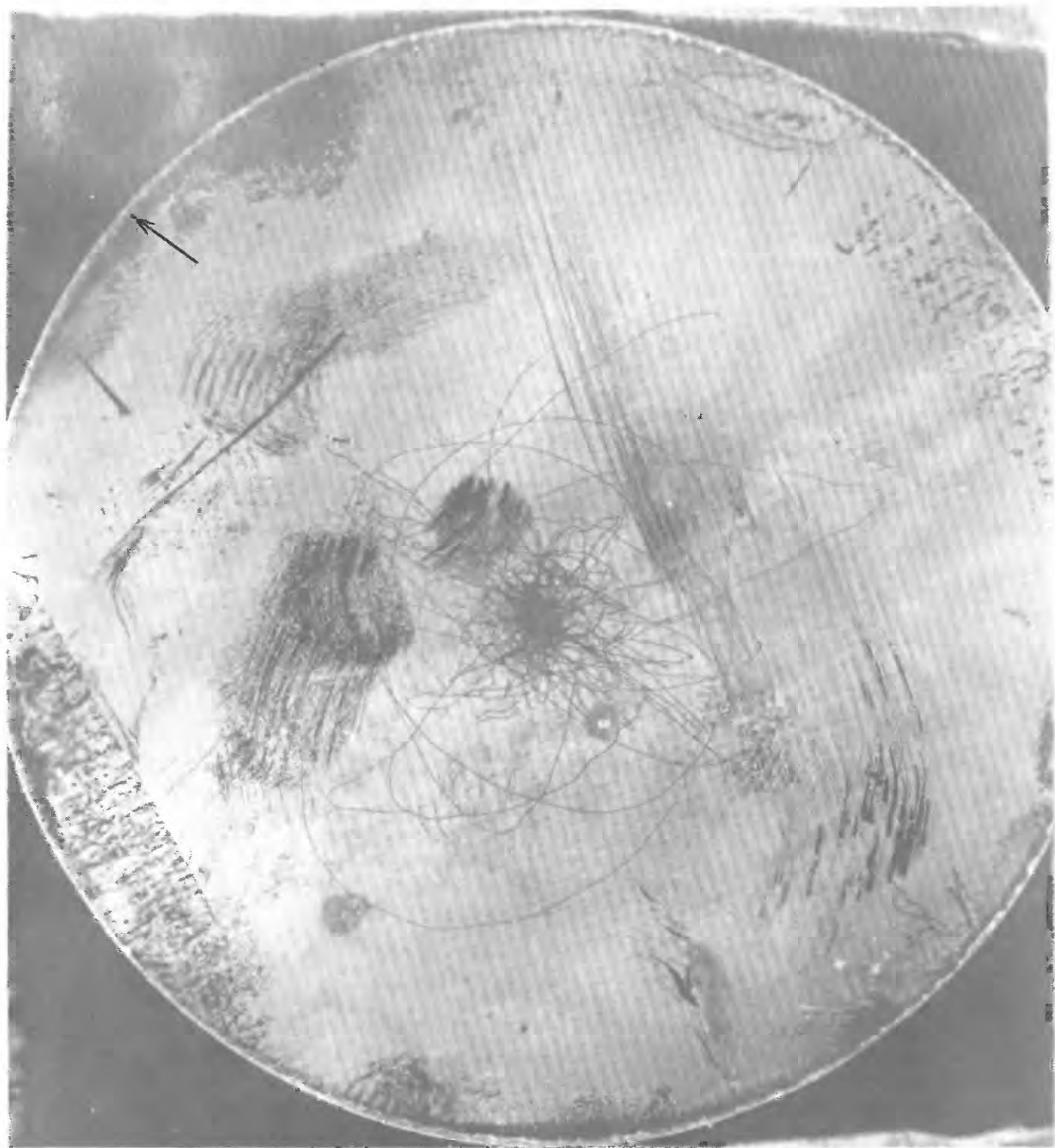
FIGURE 17.—Seismoscope plate of main event located on a ground-floor instrument at the administration building of the Universidad de San Carlos, Guatemala City. Instrument was about 30 km south of Motagua fault surface breakage. Arrow indicates north. The plate is scratched all over. Recording of main event is shown in middle part of plate.
