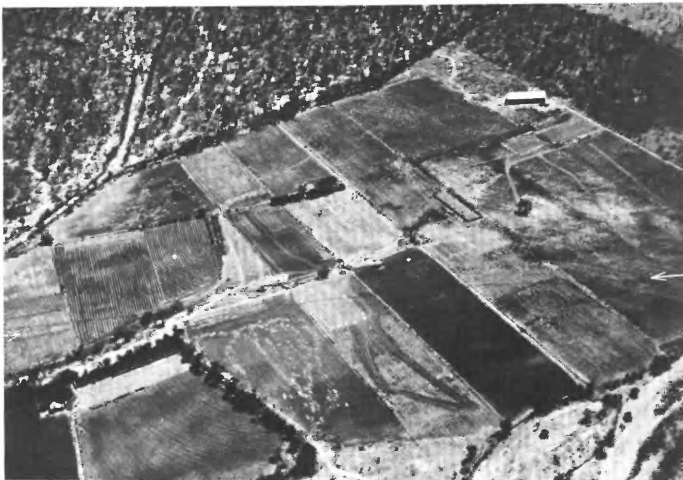
FIGURE 24.—Oblique aerial view looking south towards linear trace of the Motagua fault (arrows) in farmland west of Cabañas. Furrows with sinistral offset may be seen in the field at left. See figure 23 for location of Cabañas.
