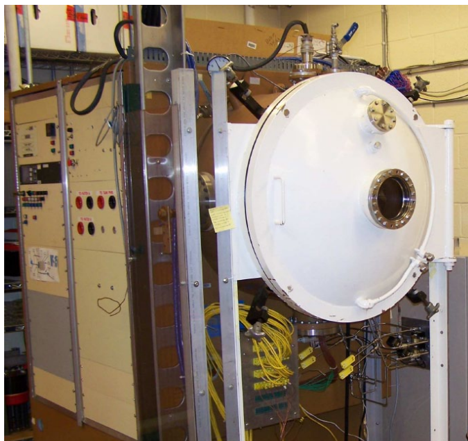
Figure 18.—Heat exchanger vacuum test chamber.
