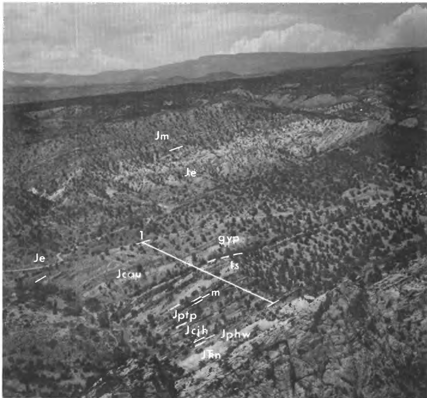
FIGURE 15.—Reference section of Carmel Formation and Page Sandstone at Pine Creek near Escalante, Utah. View is toward northwest across valley of Pine Creek. 1, reference section; Jfn, Navajo Sandstone; Jphw, Harris Wash Tongue of Page Sandstone; Jcjh, Judd Hollow Tongue of Carmel Formation; Jptp, Thousand Pockets Tongue of Page Sandstone including red marker bed shown by m; Jcau, upper member of Carmel Formation including limestone-bearing part shown by ls and gypsum-bearing part shown by gyp; Je, Entrada Sandstone; Jm, Morrison Formation. For scale, section from top of Navajo Sandstone to base of Entrada Sandstone is 162.5 m thick.
