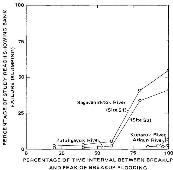
FIGURE 9.—Plot of percentage of sample sinuous or meandering reaches showing bank failure, versus percentage of time interval between breakup and peak of breakup flooding. Only partial data were collected from the Putuligayuk River.
