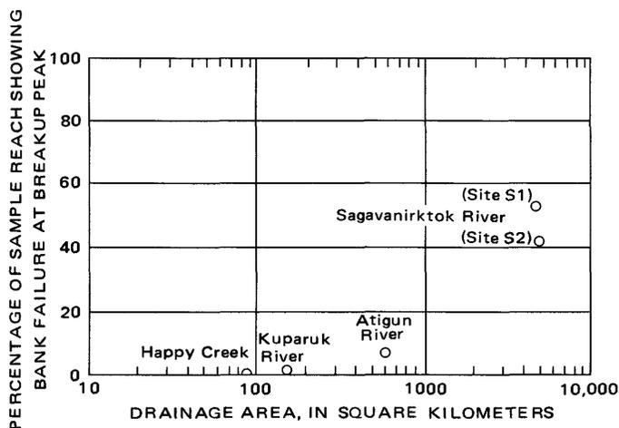
FIGURE 11.—Plot of percentage of sample reaches showing bank failure at peak of breakup flooding, versus drainage area.
