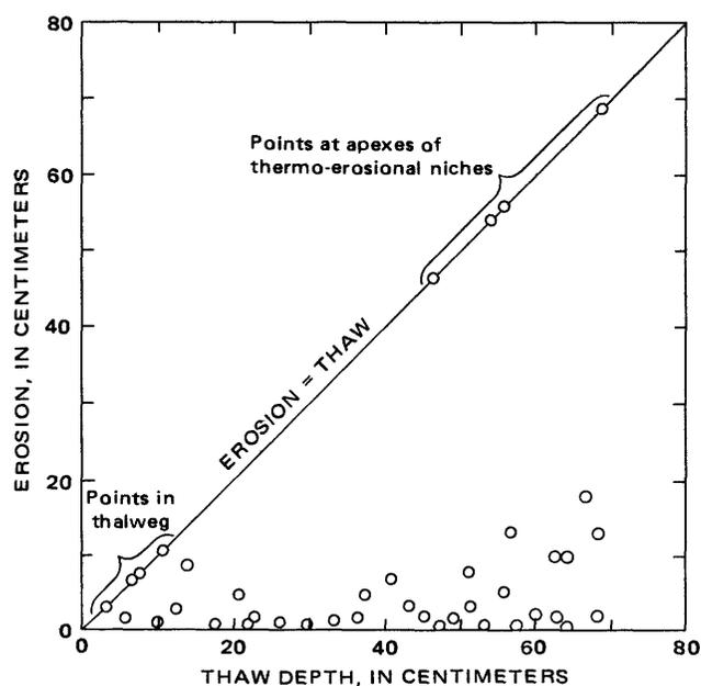
FIGURE 5.—Plot of erosion versus thaw for points in noncohesive bed and bank material. Points without detectable erosion (41) are excluded.
