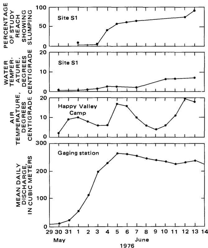
FIGURE 8.—Plot of percentage of bank failures at site S1, water temperature at site S1, maximum daily air temperature at Happy Valley Camp, and mean daily discharge at gaging station on the Sagavanirktok River. Discharge records are estimated for the period shown.
