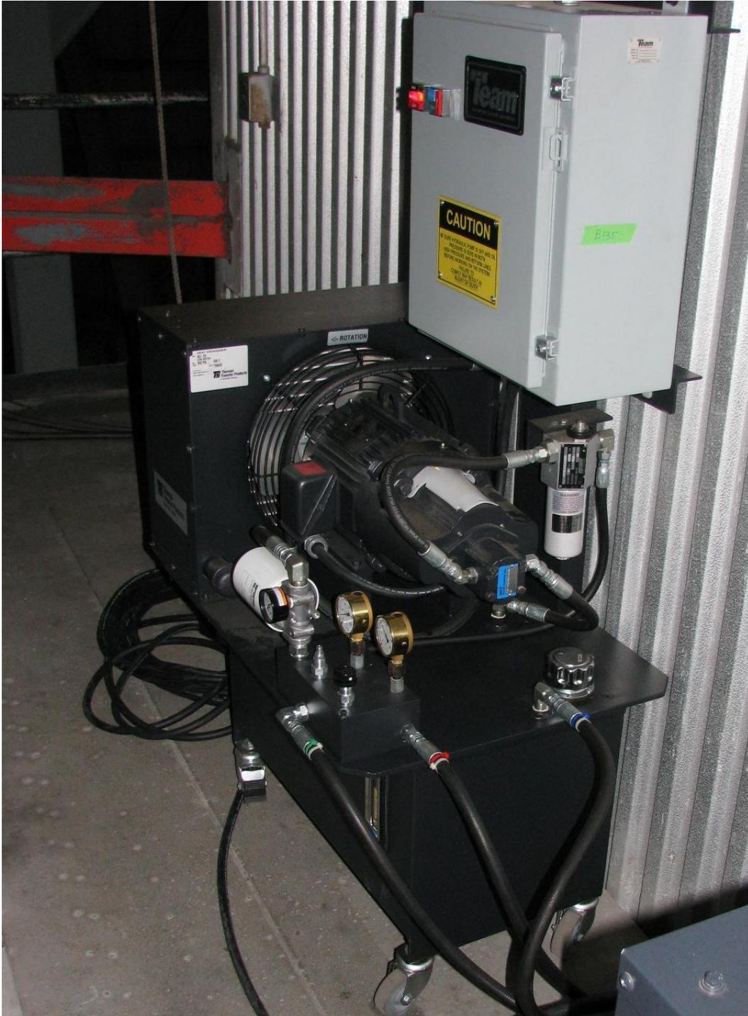
**Figure 14. Hydraulic Power Supply.**
