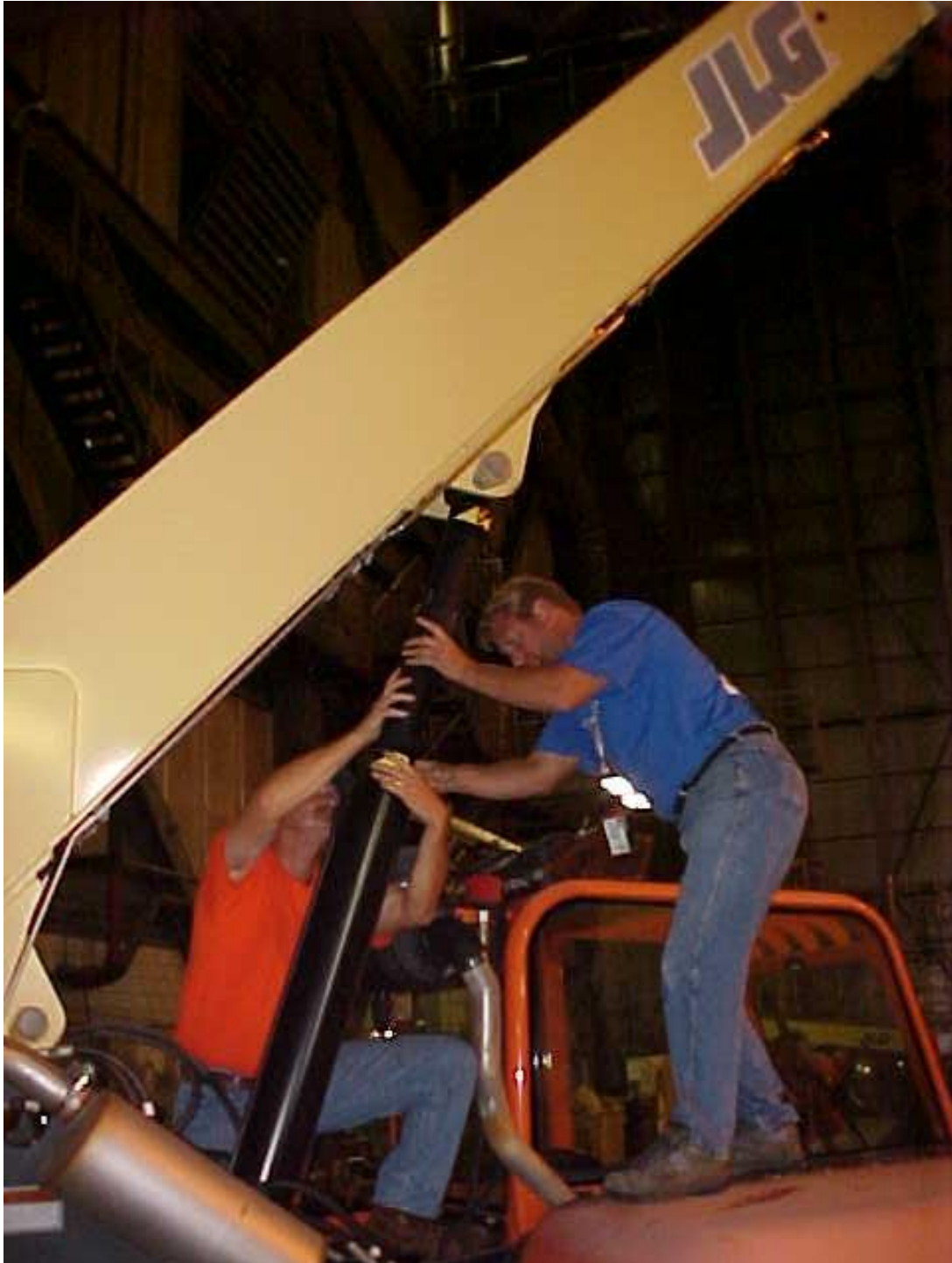
Figure 13 Installation of lockout hardware for telehandler lift
