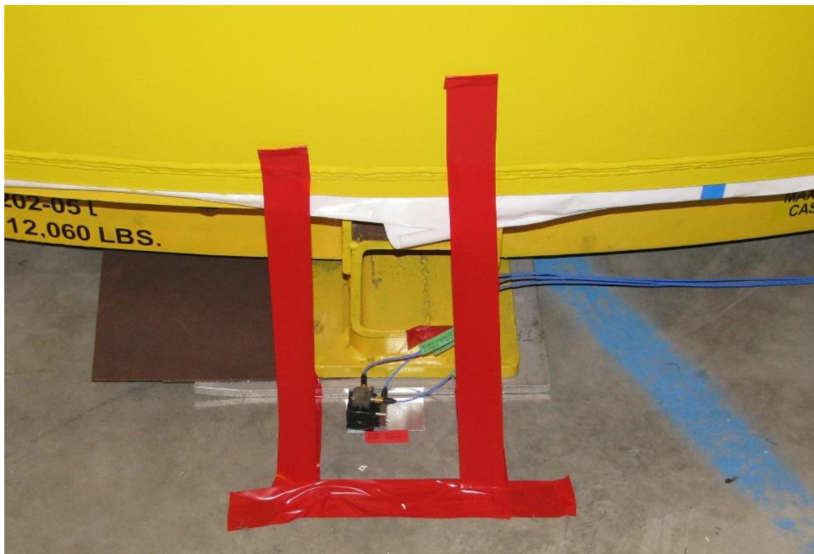
Figure 9 Shim location and ground accelerometers at 90° orientation
