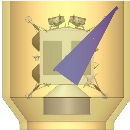
Figure 2.10—NEA Sample Return S/C—Atlas 401 Fairing Packaging Close View
