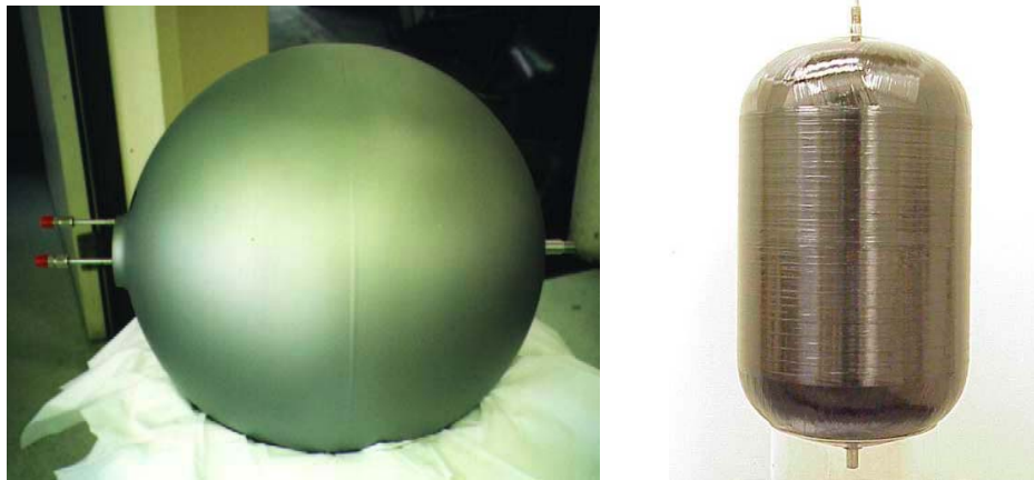
Figure 5.26—Hydrazine Tank (Left), Xe Tank (Right)
