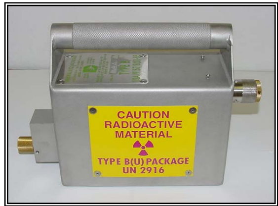
Typical radiography camera that could be stolen for illicit use
