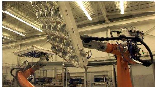
Meikle high volume automated assembly line. Top left: secondary mirrors on sheet glass. Top right: Primary mirror attachment to front glass. Bottom left: Adhesive application to primary mirrors. Bottom right: Kuka robots moving panels to next step of process.
