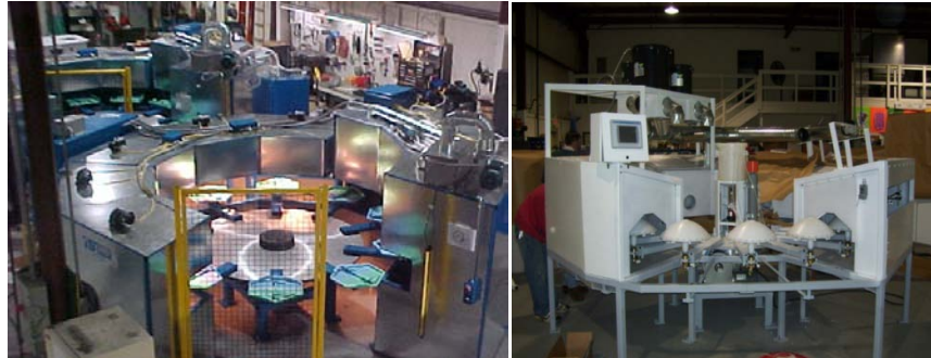
Left: Rotary batch oven. Right: Rotary coating applicator.
