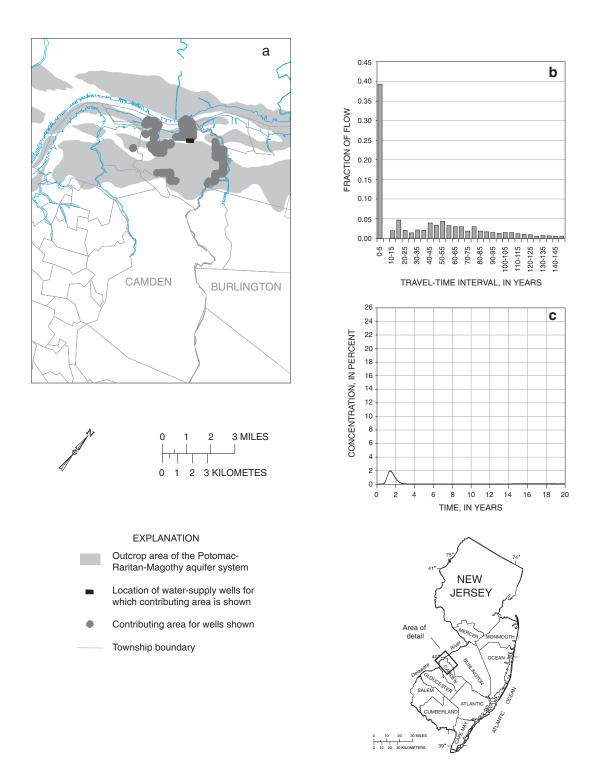
**Figure 9.** (a) Location of and contributing area for wells Morris 6, 8, and 9; (b) travel-time frequency along flow paths from the Delaware River to the wells; and (c) breakthrough concentration for a single 1-month saltwater-intrusion event.
