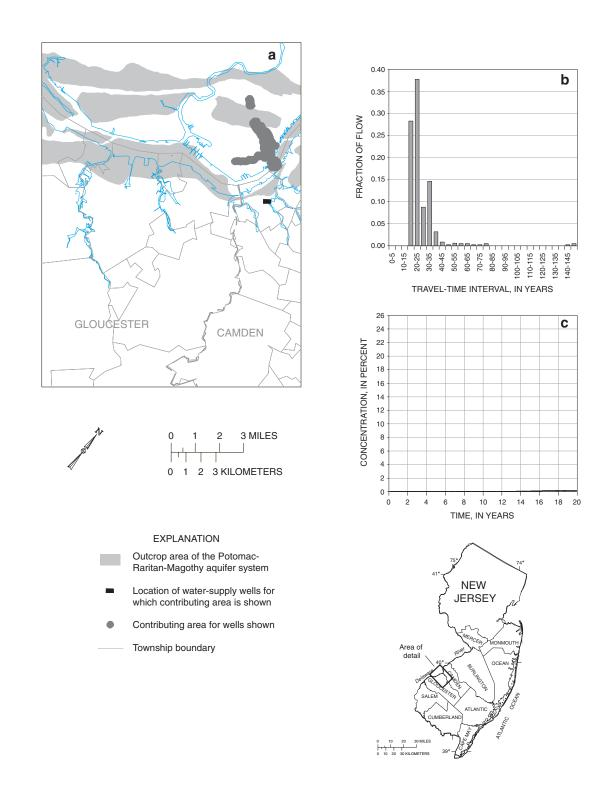
**Figure 11.** (a) Location of and contributing area for wells GCWD 40, 42, and 43; (b) travel-time frequency along flow paths from the Delaware River to the wells; and (c) breakthrough concentration for a single 1-month saltwater-intrusion event.
