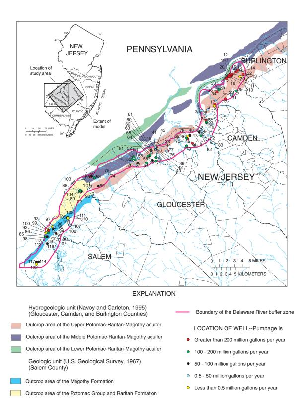
**Figure 3.** Ground-water withdrawals from wells capable of withdrawing more than 100,000 gallons per day that are within 2 miles of the Delaware River in Camden, Gloucester, and Salem Counties, N.J., 1996.
