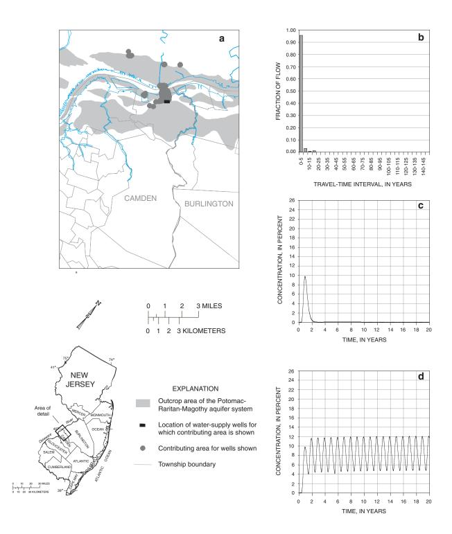
**Figure 6.** (a) Location of and contributing area for well Morris 12; (b) travel-time frequency along flow paths from the Delaware River to the well; (c) breakthrough concentration for a single 1-month saltwater-intrusion event; and (d) breakthrough concentration for an annually recurring 1-month saltwater-intrusion event.
