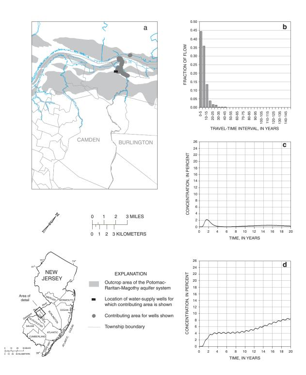
**Figure 10.** (a) Location of and contributing area for well Morris 3A; (b) travel-time frequency along flow paths from the Delaware River to the well; and (c) breakthrough concentration for a single 1-month saltwater-intrusion event; and (d) break-through concentration for an annually recurring 1-month saltwater-intrusion event.
