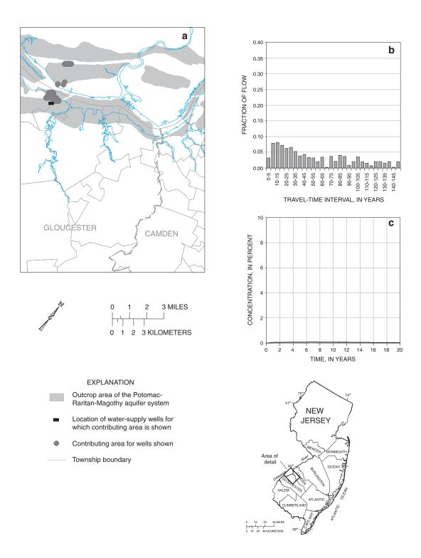
**Figure 12.** (a) Location of and contributing area for wells RW-5, RW-6, and Mobil 47; (b) travel-time frequency along flow paths from the Delaware River to the wells; and (c) breakthrough concentration for a single 1-month saltwater-intrusion event.
