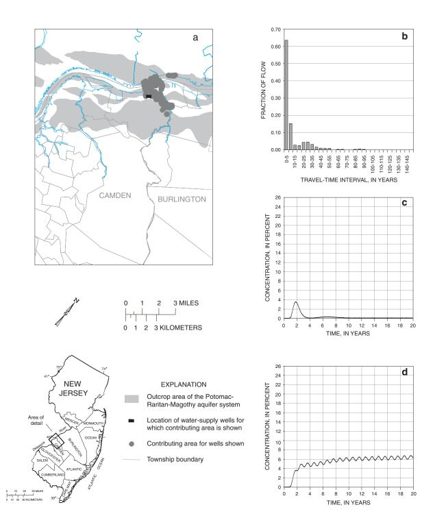
**Figure 8.** (a) Location of and contributing area for wells Morris 7 and 10; (b) travel-time frequency along flow paths from the Delaware River to the wells; (c) breakthrough concentration for a single 1-month saltwater-intrusion event; and (d) breakthrough concentration for an annually recurring 1-month saltwater-intrusion event.
