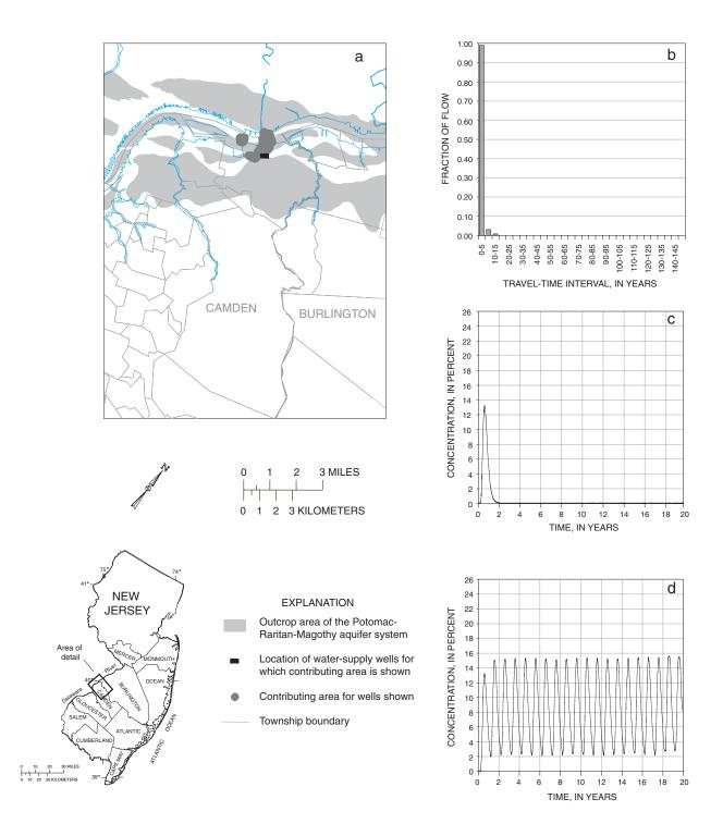
**Figure 5.** (a) Location of and contributing area for wells Morris 11 and 13; (b) travel-time frequency along flow paths from the Delaware River to the wells; (c) breakthrough concentration for a single 1-month saltwater-intrusion event; and (d) breakthrough concentration for an annually recurring 1-month saltwater-intrusion event.
