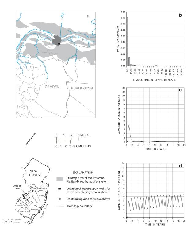
**Figure 7.** (a) Location of and contributing area for wells Delair 1, 2, and 3; (b) travel-time frequency along flow paths from the Delaware River to the wells; (c) breakthrough concentration for a single 1-month saltwater-intrusion event; and (d) breakthrough concentration for an annually recurring 1-month saltwater-intrusion event.
