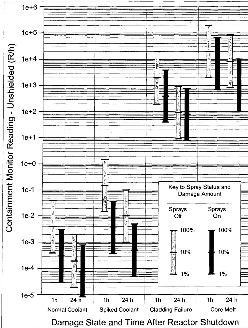
Figure 1.5 BWR Mark III Wet Well Containment Monitor Response
