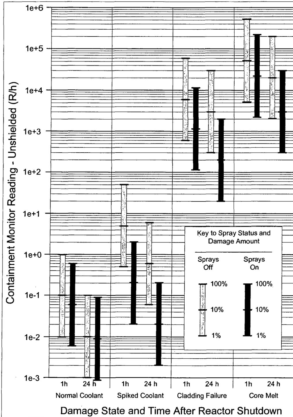
Figure 1.2 BWR Mark I and II Dry Well Containment Monitor Response
