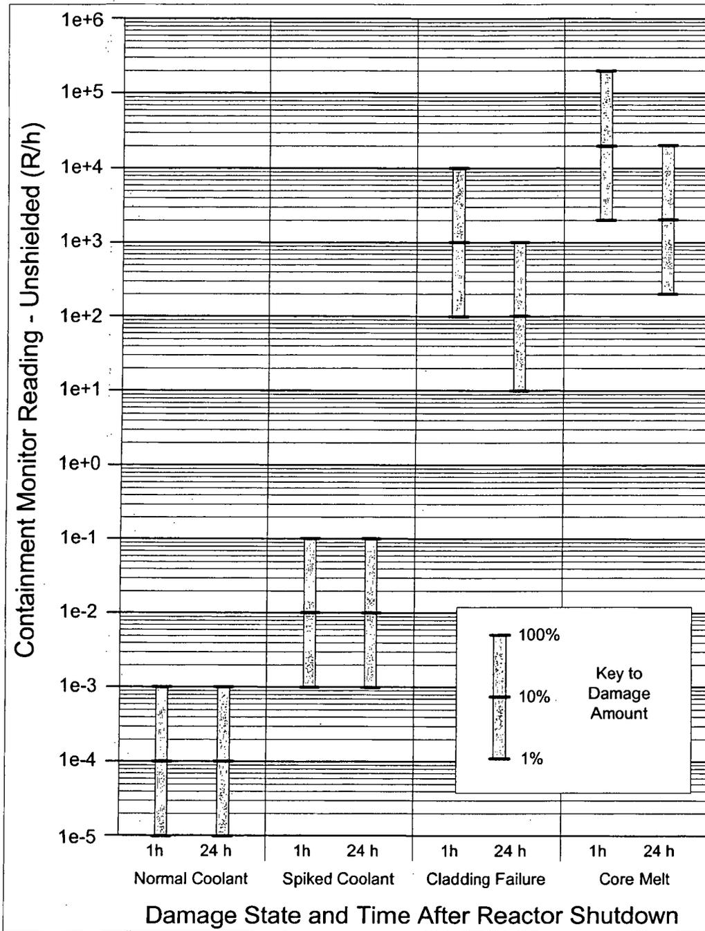
Figure 1.4 BWR Mark III Dry Well Containment Monitor Response
