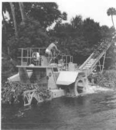
Corps tests aquatic plant harvester to control plants choking inland waterways
