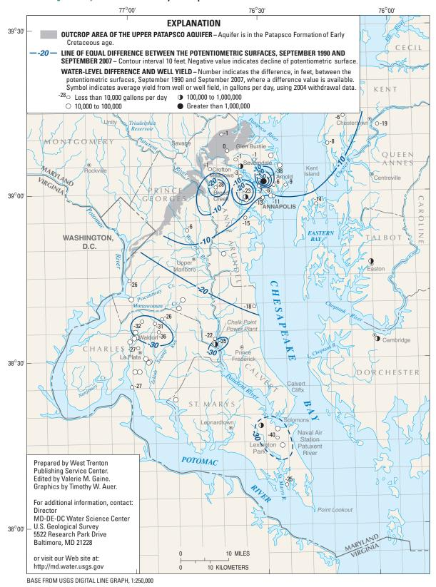
The Difference Between the Potentiometric Surfaces of the Upper Patapsco Aquifer in Southern Maryland, September 1990 and September 2007
